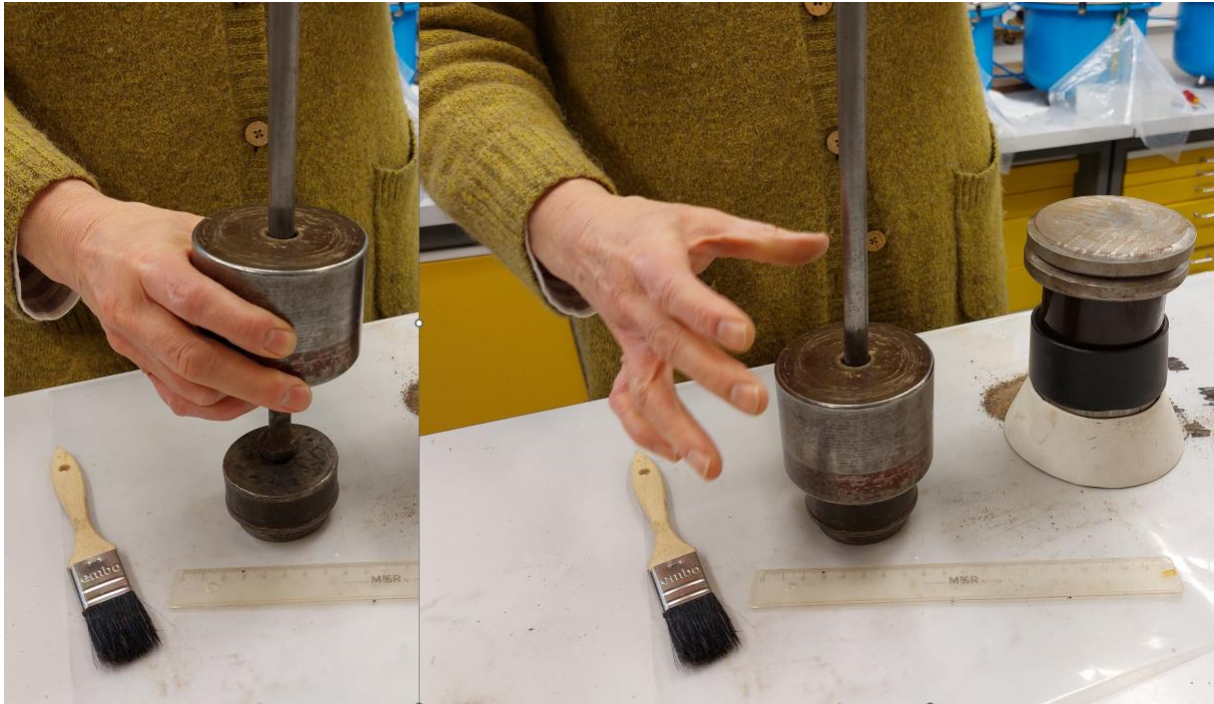
Figure 2. Packing of cylinders was done with the help of vibration generated by dropping a 2.2 kg weight for five times from a 50-mm height/JOHANNA NIKAMA
