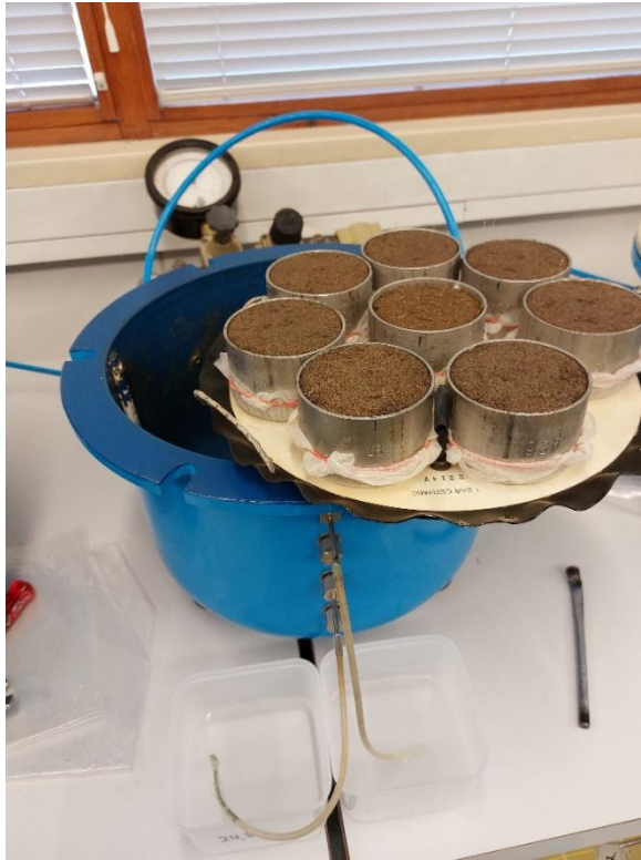
Figure 5. Cylinders on the on ceramic plates in pressure extractors on their way to pressure extractors /JOHANNA NIKAMA
